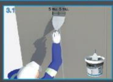
Apply RHINOZ Hybrid Jointing Compound along the joint to fill in the gap at 5 cm. width
