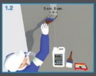
Apply RHINOZ Primer Bonding along jointing for about 5 cm. width on both sides of jointing. Leave it to dry 10–15 minutes, or until the primer bonding become clear color.
