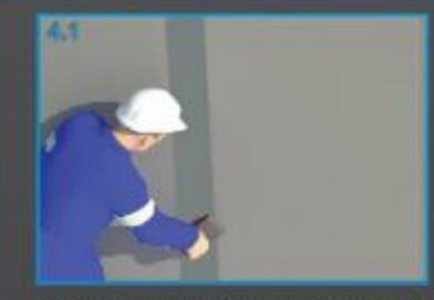
Leave it to dry completely for 24 hours. Sand the surface with sanding paper to
